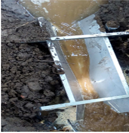
Figure 4. Infiltration measurement at plot by using double infiltrometer.
