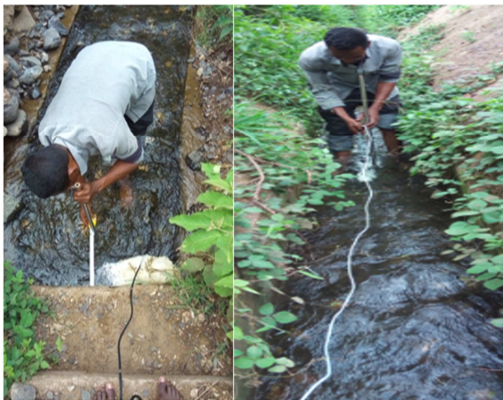
Figure 5. Flow Measurement at Main Canal by using current meter.
