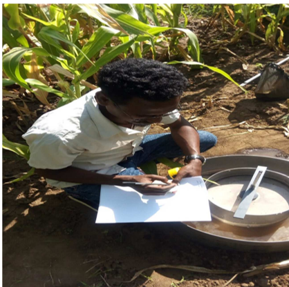
Figure 3. Infiltration measurement at plot by using double infiltrometer.
